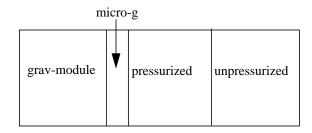
The reason for flat end caps is now clear. Since three grav-modules can fit inside the shielding, every meter the end cap deviates from a plane adds six meters of length to the shielding, and thus increases shielding mass. Flat end caps do require greater structural mass. However, shielding mass dominates the total mass of space biospheres<sup>2</sup>.
